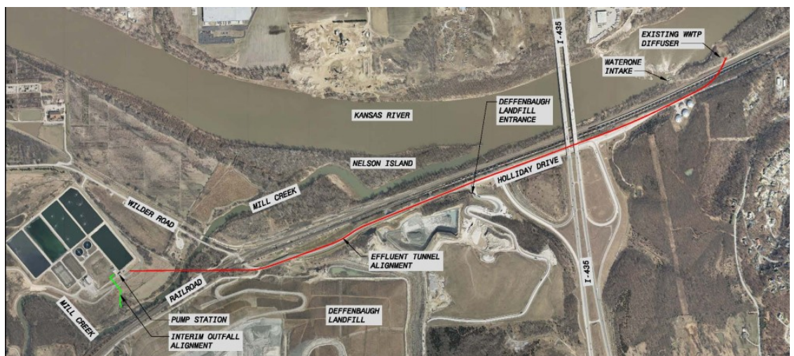
The tunnel project is shown as the red line from the treatment plant and the water intake site of Water District No. 1.
